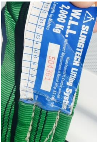
Fig 2. Shows properly rated shackle and lifting strop with tag.
