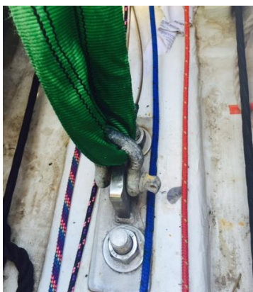
Fig 3. Shows that the vessel is securely attached at the fixed lifting points and the hook of the crane. Also correct alignment of crane to vessel.
